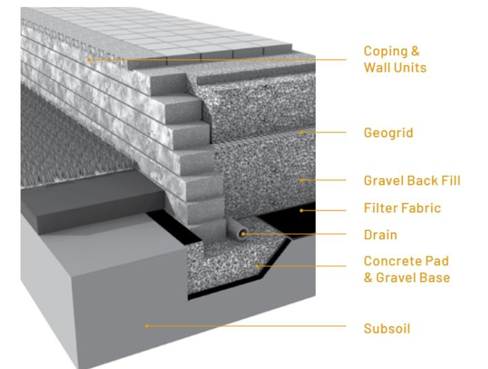
A proper base ensures that your pavers and walls won't shift during freeze/thaw cycles.
